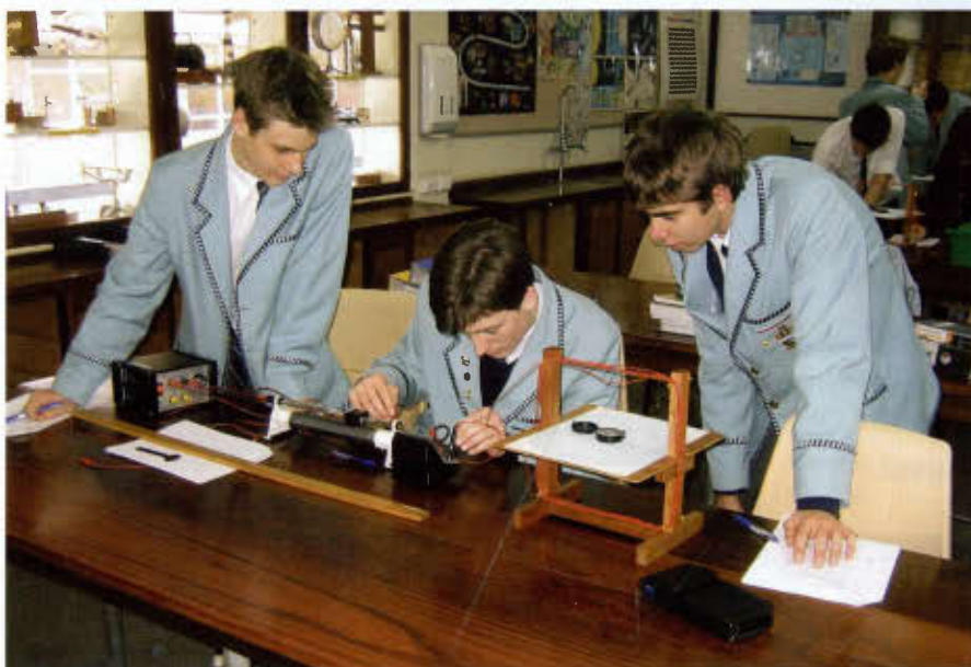
Year 12 students Chris Marr, Thomas Jelenich and Daniel Jenkins measure the angular deviation produced by the magnetic field associated with electric current flowing in a coil.
